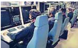
The 9SCS Mark 3 Combat Management System has three multifunction consoles.
